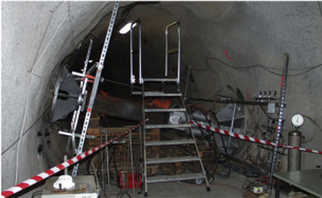
Figure 5 - The plate load apparatus assembled for a long-term test in an underground rock laboratory in Switzerland. The metal frame to hold the displacement transducers measuring the plate movement can be recognized on both sides of the tunnel.
